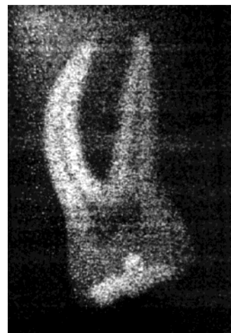
Figure 17. Latent X-ray image of a tooth in a Yb–Tm-doped vitrocereamic, revealed by the blue emission under an IR irradiation at 960 nm.
